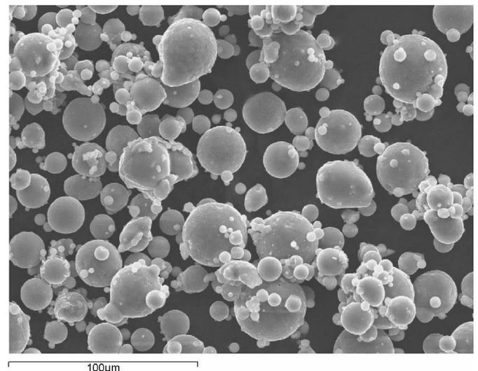
**Fig. 1.** SEM image of the AlSi10Mg alloy powder.
