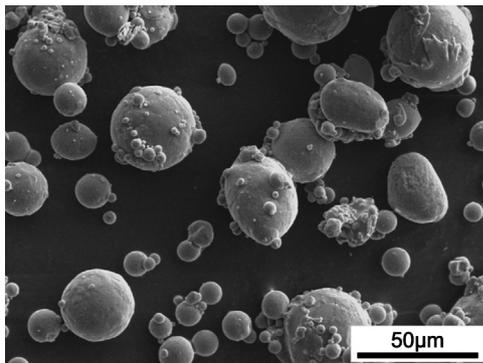
Fig. 1. Scanning electron micrograph of the Al–12Si powder used.
