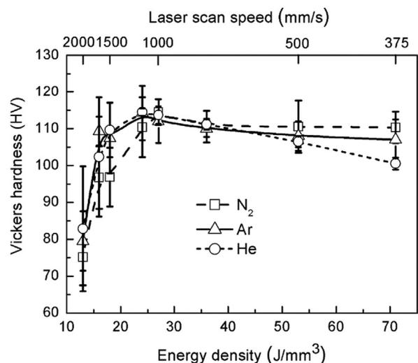
Fig. 4. The effect of laser energy density on the hardness of SLM-produced Al–12Si in Ar, N<sub>2</sub> and He atmospheres. Similar to Fig. 2, the hardness increases with energy density and there is no significant difference between atmospheres. Individual points are an average of 12 tests. Error bars show one standard deviation.
