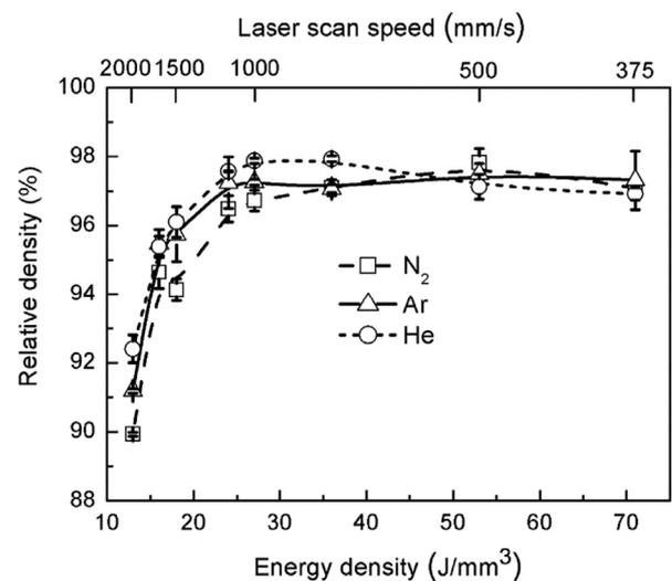
Fig. 3. Relative density of the SLM-produced Al–12Si samples as a function of incident laser energy. There is a general trend of increasing density with laser energy density, up to  $\sim 30$  J/mm<sup>3</sup>, after which the density plateaus. There is no significant difference between the three atmospheres. Individual points are an average of 3 tests and error bars show one standard deviation.
