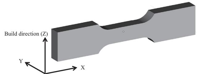
Fig. 2. Orientation of the tensile bar relative to the building direction.
