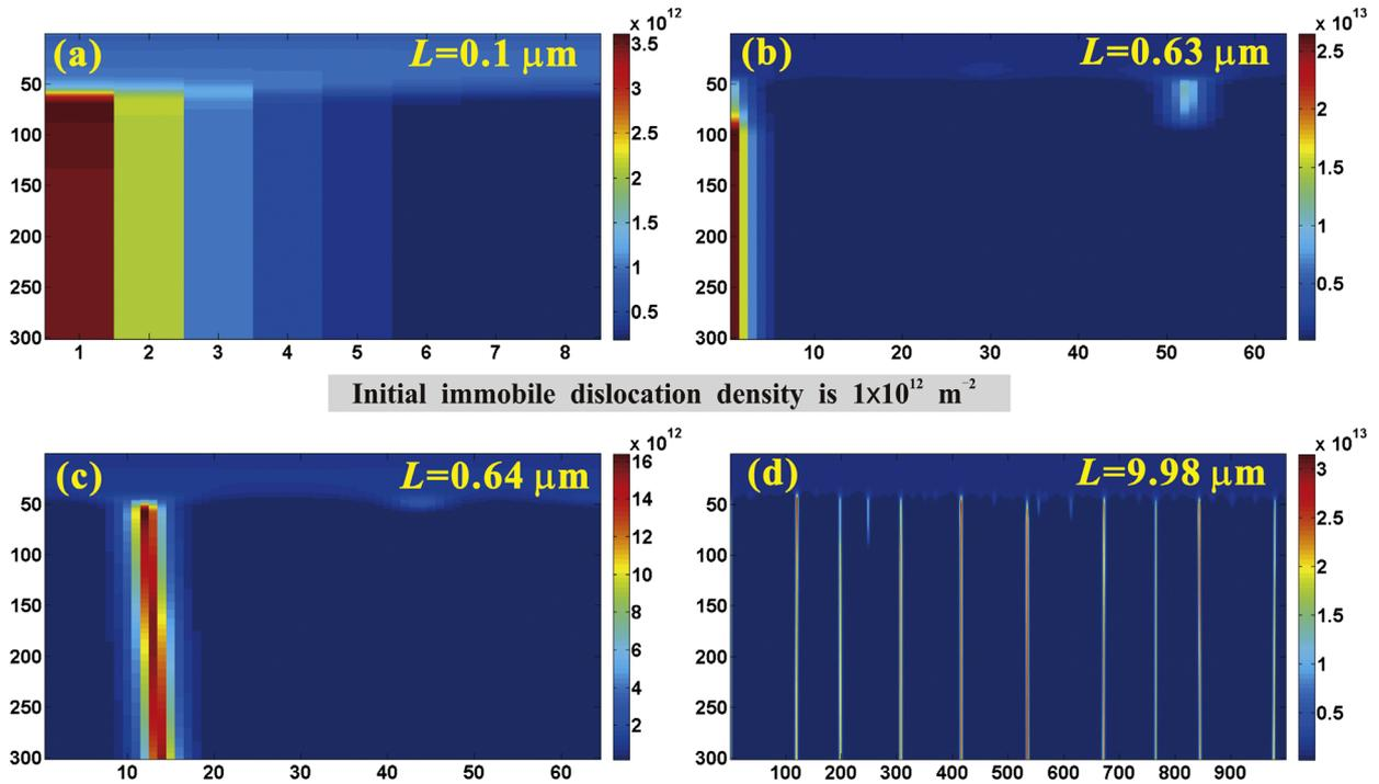
Fig. 1. Dislocation patterning behavior inside the grains with a size of  $L =$  (a) 0.08, (b) 0.63, (c) 0.64, and (d) 9.98  $\mu\text{m}$  for a given  $\rho_{\text{IDD}} = 1 \times 10^{12} \text{ m}^{-2}$ , respectively. The Y axis indicates nominal fatigue cycles and the X axis refers to the location for dislocation patterning.
