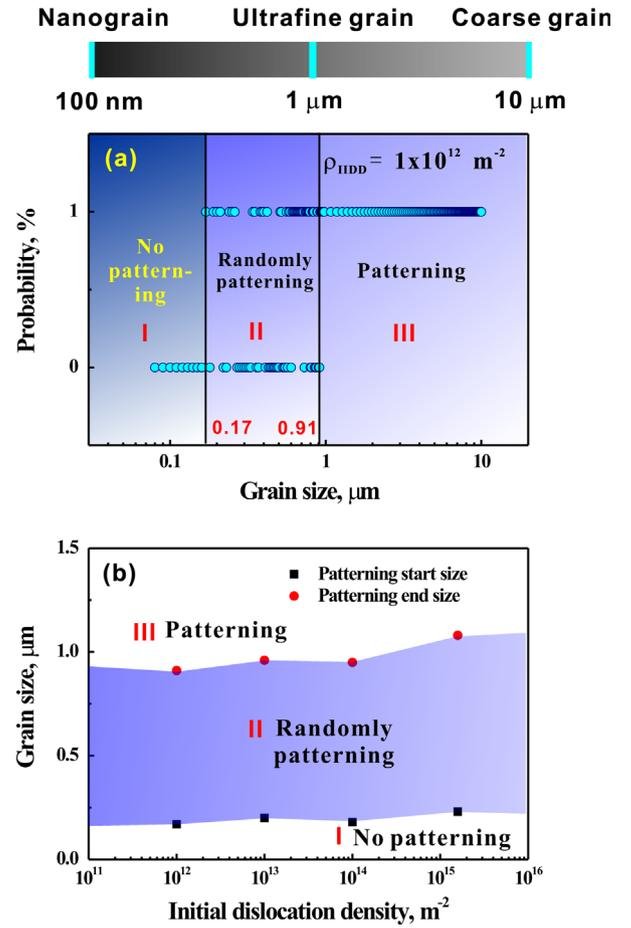
Fig. 2. (a) Possibility of dislocation patterning as a function of grain size with  $\rho_{\text{IDD}} = 1 \times 10^{12} \text{ m}^{-2}$ , (b) relationship between the dislocation patterning-needed (DPN) grain size and the initial immobile dislocation density.
