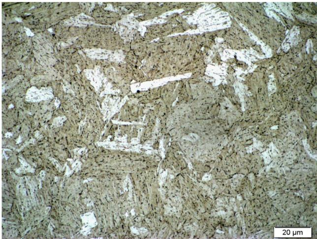
Fig. 1. BA-160 base metal microstructure.
