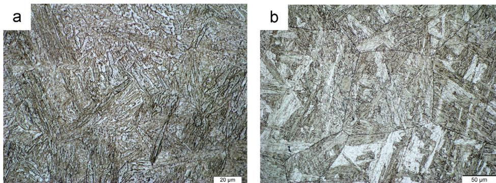
Fig. 2. Optical micrographs for the BA-160 CGHAZ: (a) as-welded and (b) after PWHT.
