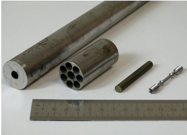
Fig. 1. Extraction of miniature creep specimens from a superheater tube for steam power plants. The tube (left) is cut into 60 mm long sections which allow extracting bars of 7 mm diameter out of the sidewall by electrical discharge machining. From these pieces, cylindrical creep specimens (right) are machined according to Fig. 2.
