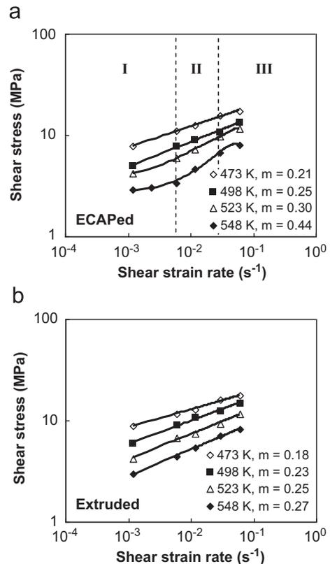
Fig. 2. Shear stress as a function of shear strain rate for (a) ECAPed, and (b) extruded conditions at various temperatures.
