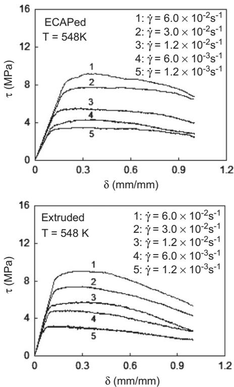
Fig. 1. SPT curves of the material obtained at different strain rates and  $T=548$  K.
