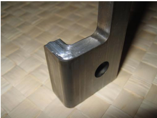
Fig. 2. Material pickup on the bottom surface of a 3D-ECAP channel.
