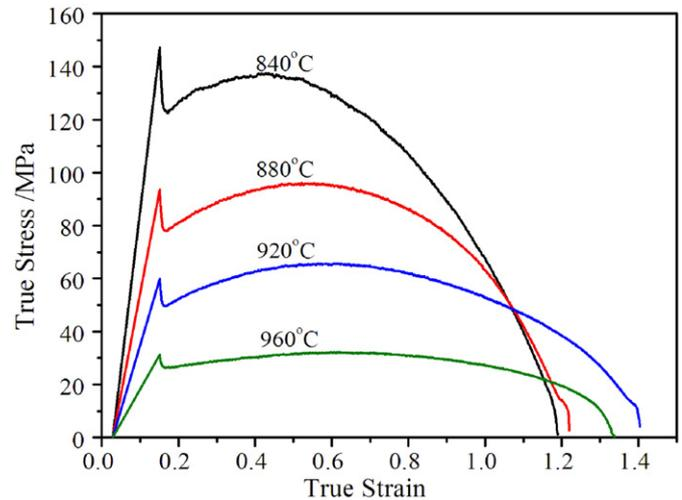
Fig. 3. True stress-true strain curves of Ti600 alloy during tensile tests.
