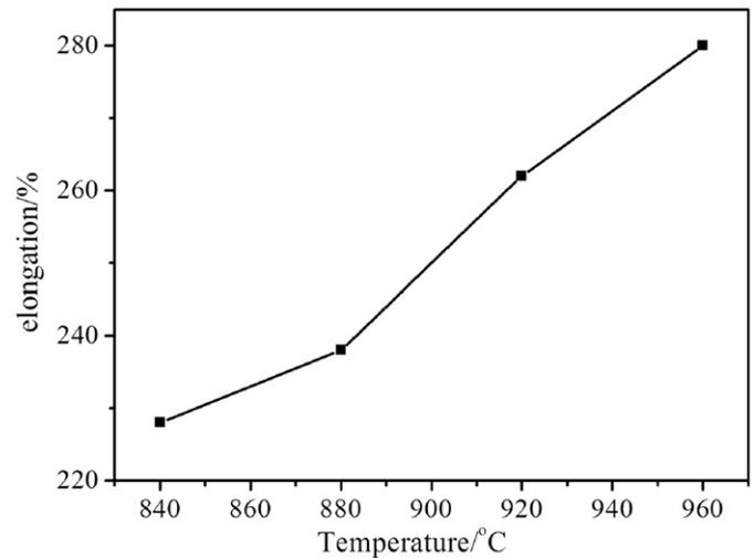
Fig. 4. Effect of temperature on elongation of Ti600 alloy.
