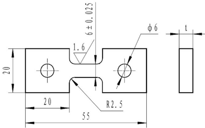
Fig. 1. Schematic diagram of specimens for superplastic tensile test.
