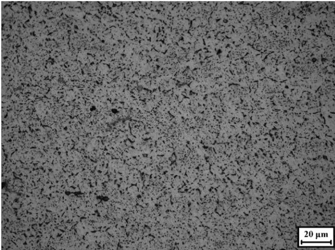
Fig. 2. Microstructure of as-received specimen of Ti600 alloy.
