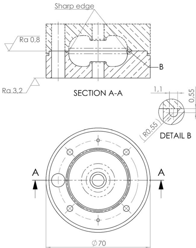
Fig. 1. Brazing surface and cross section of the cavity A (dimensions are in mm).
