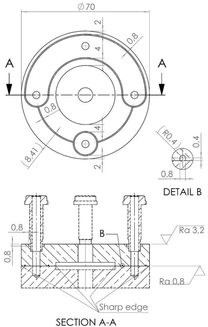
Fig. 2. Brazing surface and cross section of the cavity B and connectors for the cooling circuit (dimensions are in mm).
