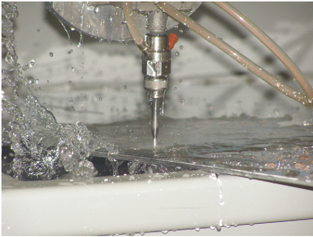
Fig. 1. Close up of a typical abrasive waterjet head.
