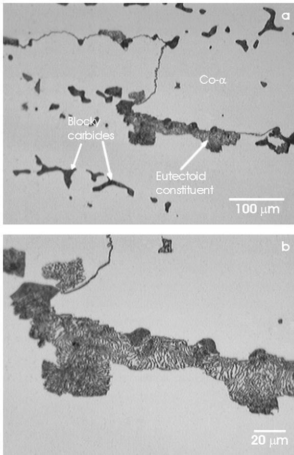
Fig. 1 – As-cast microstructure of the ASTM F75 alloy.
