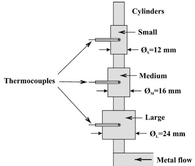
Fig. 2 – Schematic illustration of the casting arrangement.
