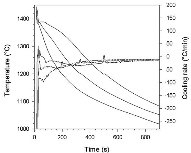
Fig. 3 – Typical cooling curves and their derivatives obtained by thermal analysis of the ASTM F75 alloy. Cooling curves from casting A1-2, 0.26 wt.% carbon.
