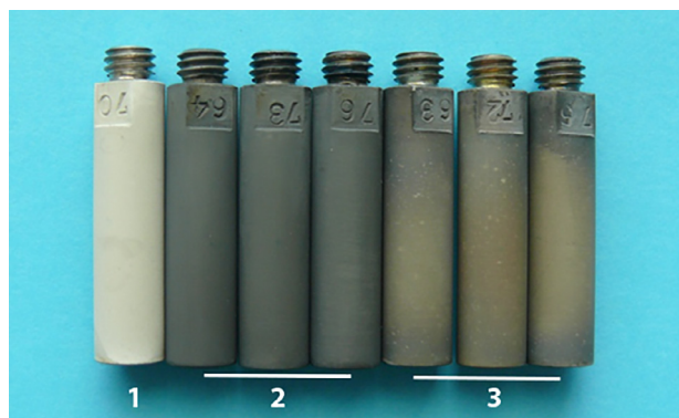
Fig. 1. Fabricated corrosion test samples of Eurofer after different fabrication steps: As coated (1), after 1 st HT step (2) and after the 3 rd HT step (3).
