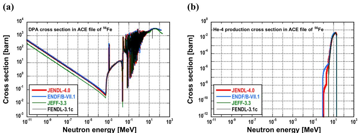
Fig. 2. (a) DPA cross section, (b) He-4 production cross section of  $^{56}\text{Fe}$ .
