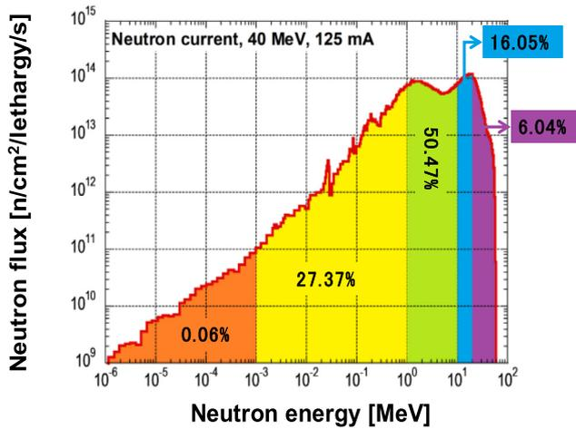
Fig. 1. Calculated A-FNS neutron spectrum behind the back plate.
