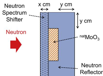
Fig. 3. Calculation model of RI module.  $x$  cm is thickness of neutron spectrum shifter and  $y$  cm is thickness of reflector.
