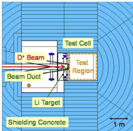
Fig. 2. Calculation model on test cell in A-FNS.
