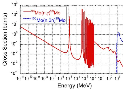
Fig. 1. Cross sections of  $^{99}\text{Mo}$  production.
