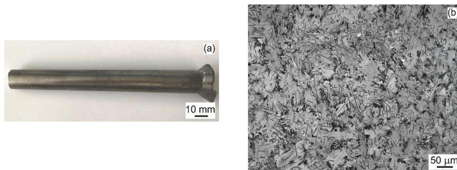
Fig. 1. OM micrographs of centrifugally cast in-situ composite: (a) as-cast conical sample with a feeding head; (b) transverse section showing equiaxed grain microstructure.
