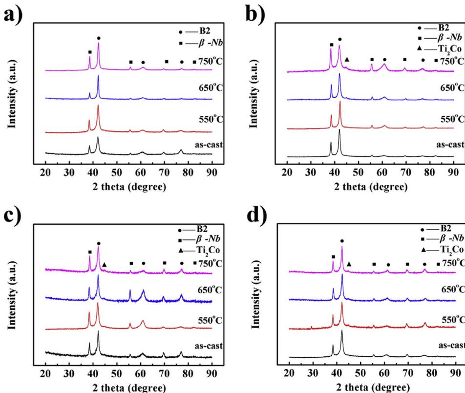
Fig. 1. Room temperature XRD profiles of the as-cast and annealed  $\text{Ti}_{44.5}\text{Ni}_{46.5-x}\text{Nb}_9\text{Co}_x$  ( $x = 0.5, 1, 2, 4$ ) alloys, (a) 0.5Co, (b) 1Co, (c) 2Co, (d) 4Co.
