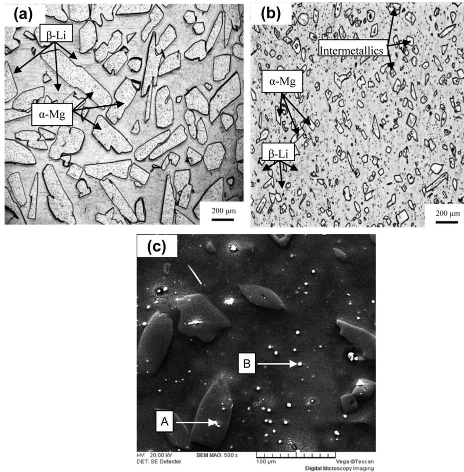
Fig. 1. Microstructures of (a) the as-cast Mg-9Li alloy, (b) the as-cast Mg-9Li-0.3Y alloy, and (c) SEM images of the as-cast Mg-9Li-0.3Y alloy.
