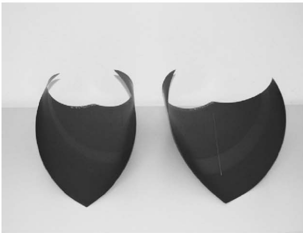
Fig. 1. Multistable deformation states of unsymmetric composites.
