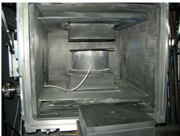
Fig. 1. Reaction chamber of a FAST/SPS sintering press adapted for the measurements.
