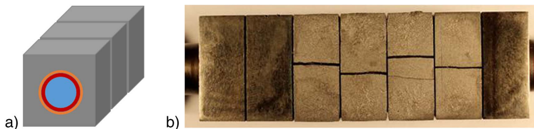
Fig. 1. a) Schematic view of a tungsten monoblock mock-up consisting of a CuCrZr-tube with 12 mm inner diameter and a thickness of 1.5 mm, a 1 mm pure copper interlayer and surrounding tungsten blocks with 28 \times 12 mm front surface and a varying height (plasma front thickness 5.5 to 8 mm); b) Top view of such a mock-up with 7 tungsten blocks after testing at 20 \text{ MW/m}^2 .
