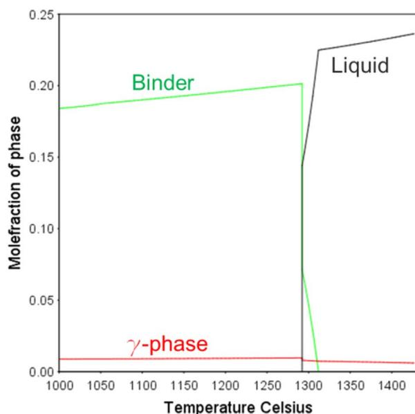
Fig. 1. Mole fractions of binder,  $\gamma$ -phase and liquid versus temperature.
