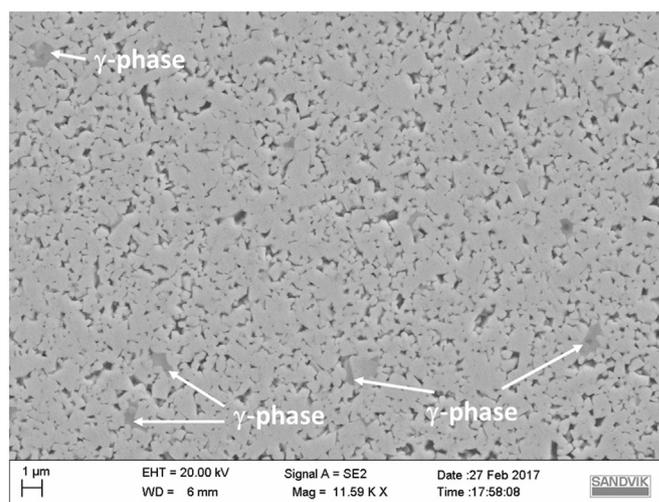
Fig. 2. SE SEM image of the Ti containing WC-Co revealing grey regions assumed to be  $\gamma$ -phase beside WC grains (light grey), Co rich binder phase areas (darker areas).
