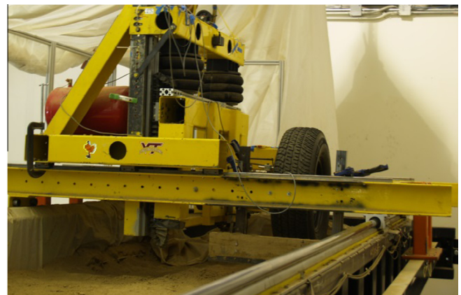
Fig. 1. Terramechanics Rig filled with silty sand and fitted with off-road tire.
