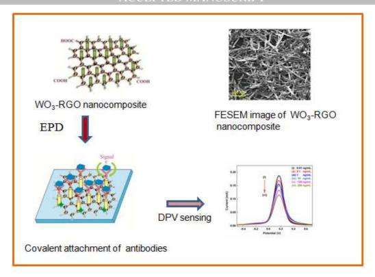
The proposed WO<sub>3</sub>-RGO nanocomposite based immunosensor exhibited a high sensitivity and much broader detection range for cTnI cardiac biomarker
