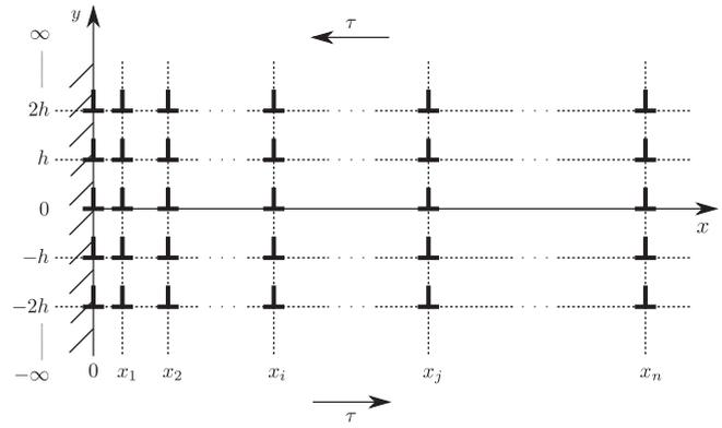
Fig. 1. Pile-up of vertical walls of edge dislocations in an infinite elastic medium. The dislocation wall at  $x=0$  is immobile.
