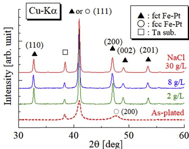
**Fig. 2.** XRD patterns of the as-plated Fe<sub>50</sub>Pt<sub>50</sub> film for NaCl = 30 g/L and the annealed ones for NaCl = 2, 8, and 30 g/L.
