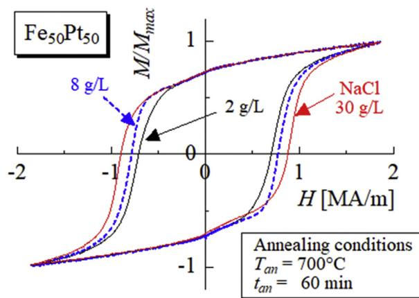
**Fig. 1.** Hysteresis loops of the annealed Fe<sub>50</sub>Pt<sub>50</sub> films prepared at NaCl = 2, 8, and 30 g/L.
