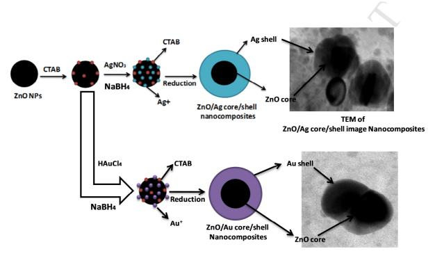
TEM of ZnO/Au core/shell image Nanocomposites
