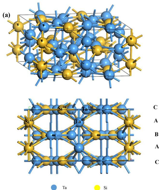
Fig. 1. Crystal structures (a) and atomic arrangement on (010) plane (b) for the D8<sub>m</sub>-structured  $\beta$ -Ta<sub>5</sub>Si<sub>3</sub> crystal structure.
