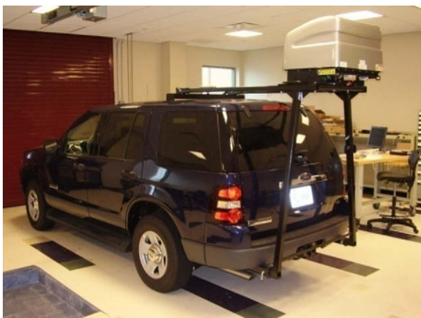
Fig. 1. Host vehicle with attached Vehicle Terrain Measurement System.
