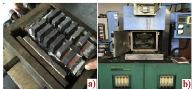
Fig. 3. a) Taking the samples into the sintering mold b) Sintering machine.
