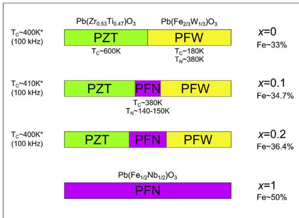
Fig. 1. The schematic diagram illustrating the main motivation of the work. \* - data from work [26].
