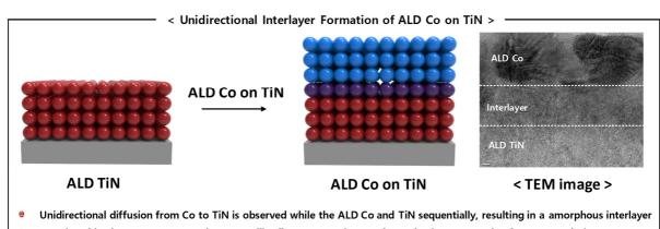
By using this phenomenon, amorphous metallic alloy, ALD CoTiN, was formed using supercycle of ALD Co and TiN
