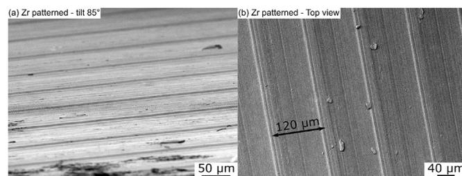
Fig. 1. SEM images of the surface of zirconium patterned with an array of 1 μm-high ridges spaced every 120 μm. (a) tilt 85°. (b) Top view.
