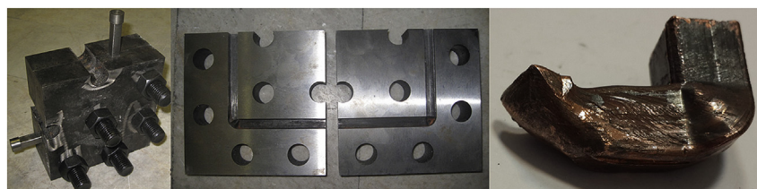
Fig. 2. The utilized PTCAE die and deformed copper sample after the first pass.
