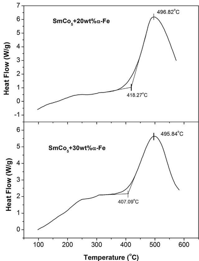
Fig. 2. The DSC curves of as-milled  $\text{SmCo}_5 + x\text{wt}\%$  ( $x = 20, 30$ ) samples.
