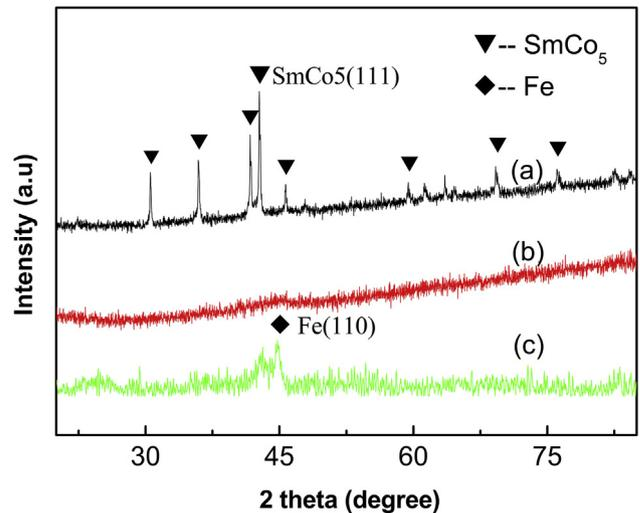
Fig. 1. The XRD patterns of (a) Sm–Co powders before milling, (b) as-milled  $\text{SmCo}_5 + 20$  wt.%  $\alpha\text{-Fe}$  sample, (c)  $\text{SmCo}_5 + 20$  wt.%  $\alpha\text{-Fe}$  sample milled for 5 h and subsequent annealed at  $500^\circ\text{C}$  for 1 h under a magnetic field.
