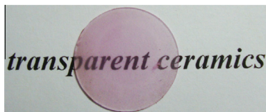
Fig. 1. Photograph of \text{Cr}:\alpha\text{-Al}_2\text{O}_3 transparent ceramics doped with 0.1 wt% \text{Cr}_2\text{O}_3 (1.20 mm in thickness).
