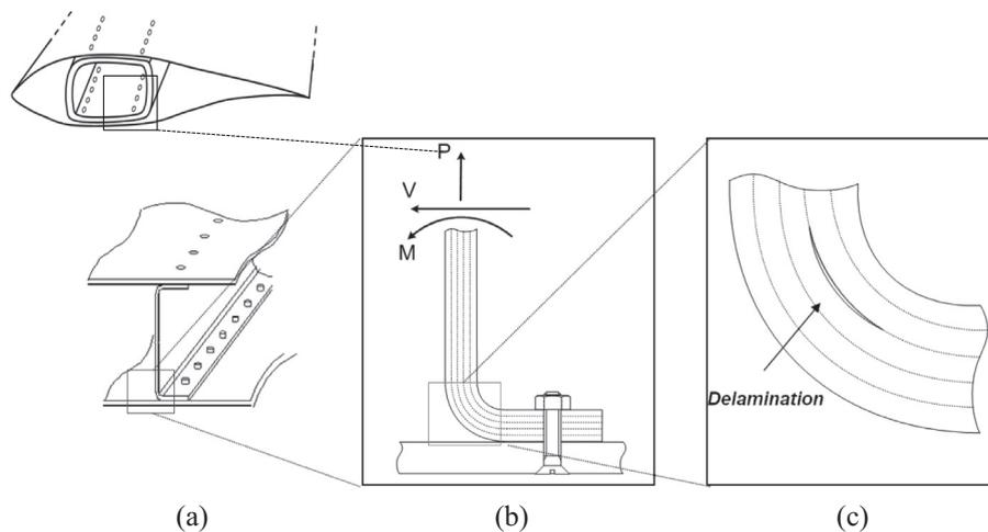
**Fig. 1.** (a) An example of an orthogonal structure in a wind turbine box and a wing spar/skin joint assembly with (b) the L-shaped laminate showing the section loads and (c) a delamination in the curved region.
