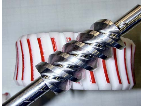
Fig. 1. Worm gear set with a non-90° crossing angle.
