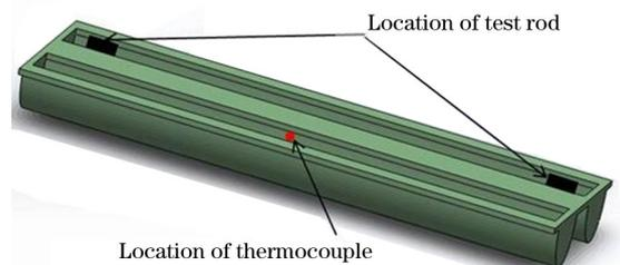
**Fig. 2.** Schematic diagram of the crucible.
