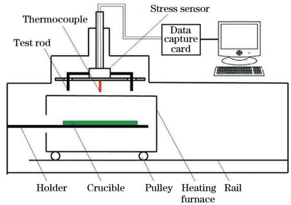
**Fig. 1.** Schematic diagram of the testing apparatus.
