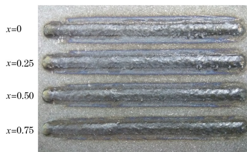
Fig. 1. Macro-morphology of the cladding layer.
