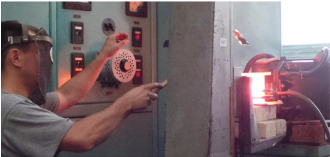
Fig. 1. Induction heating with high frequency currents in the shield gas.
