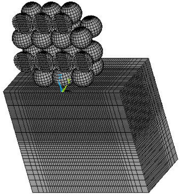
Fig. 1. 3D SP model for homogeneous materials.
