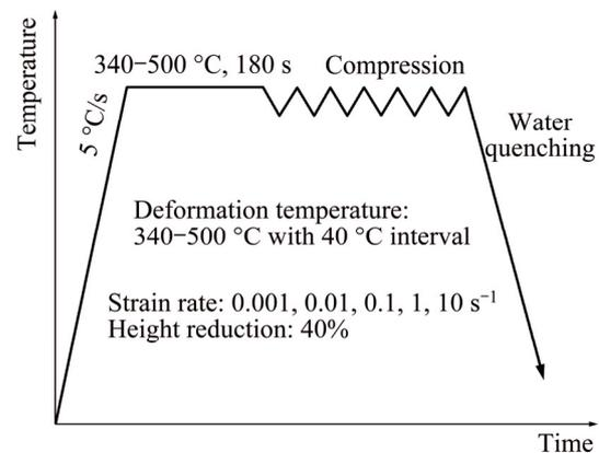
**Fig. 2** Schematic diagram of hot compression test
