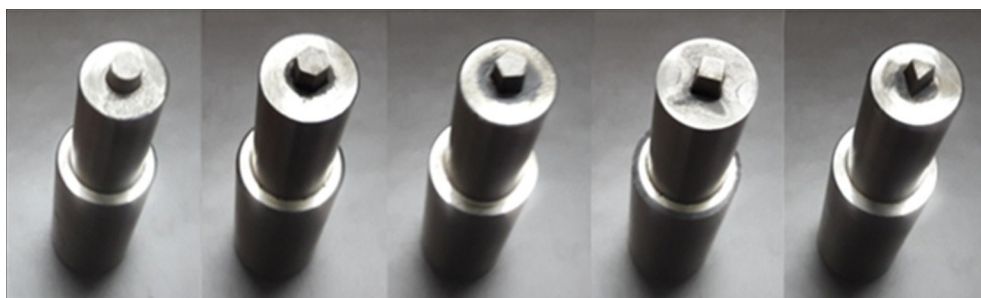
Fig. 1 Various tool pin profiles used for welding study
