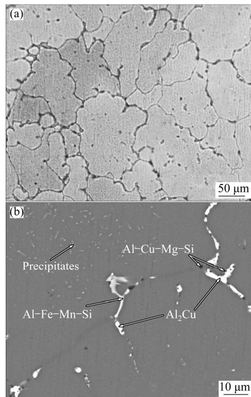
**Fig. 1** Initial microstructures of AA2014 aluminum alloy: (a) OM; (b) SEM
