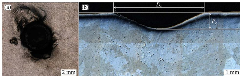
**Fig. 1** Macroscopic views of crater in depleted uranium target impacted by steel projectile at velocity of 50 m/s: (a) Top view; (b) Corresponding cross-section view
