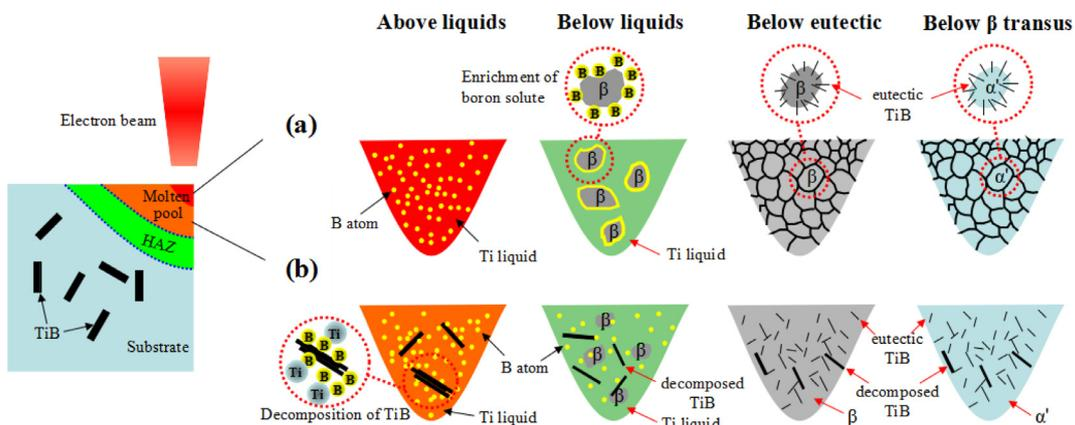
Fig. 2. Schematics illustrating formation of the remelted layer: (a) high temperature region (b) low temperature region.
