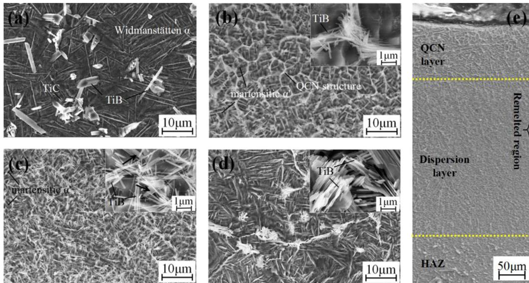
Fig. 1. Microstructure of TiB-TMCs before and after electron beam remelting: (a) un-remelted sample (b) QCN layer (c) dispersion layer (d) HAZ (e) cross section.
