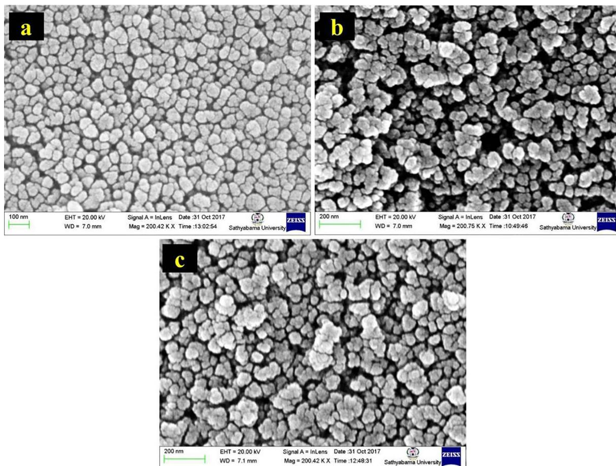
Fig. 1. FE-SEM images of (a)  $\text{TiO}_2$ , (b)  $\text{TiO}_2/\text{un-doped CdS}$  (c)  $\text{TiO}_2/2\% \text{ Pb-doped CdS QDs}$ .
