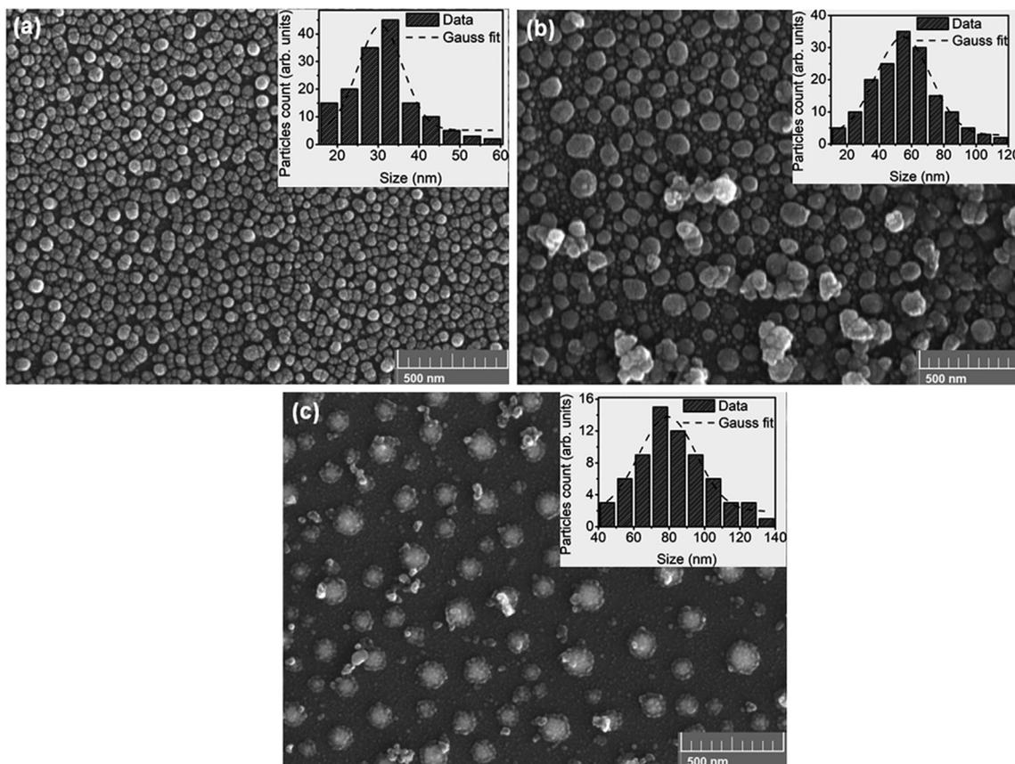
**Fig. 1.** SEM images of GaAs nanostructures irradiated with ion fluences of (a)  $1 \times 10^{13}$  ions/cm<sup>2</sup>, (b)  $5 \times 10^{14}$  ions/cm<sup>2</sup> and (c)  $5 \times 10^{15}$  ions/cm<sup>2</sup>. The size distribution of nanostructures is shown in inset.
