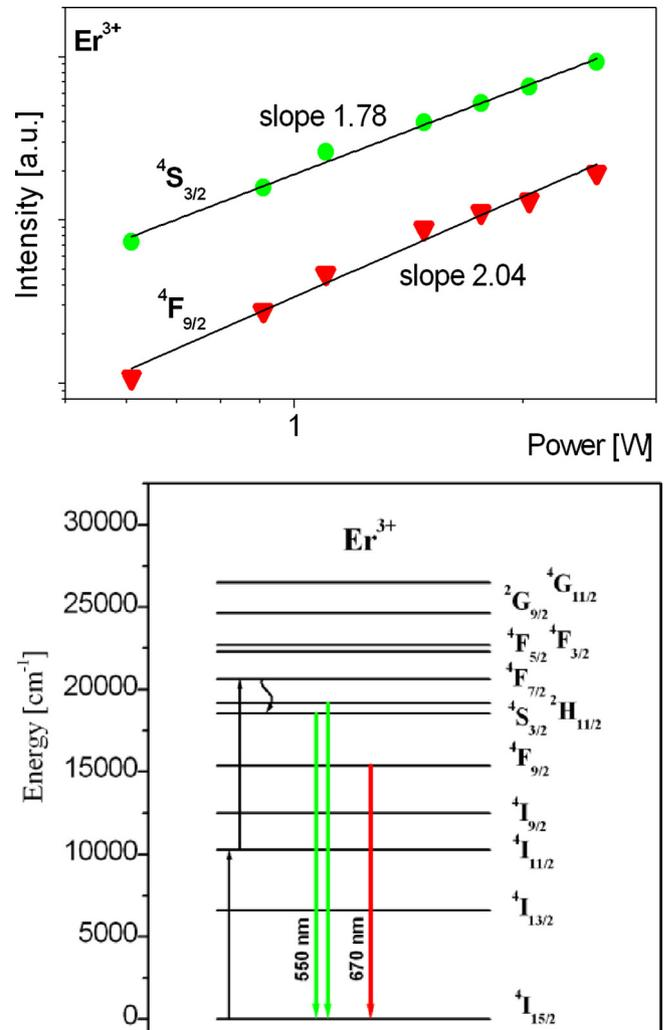
Fig. 2. The log-log dependence of up-conversion emission intensity on the excitation power (top) and the energy scheme (bottom).
