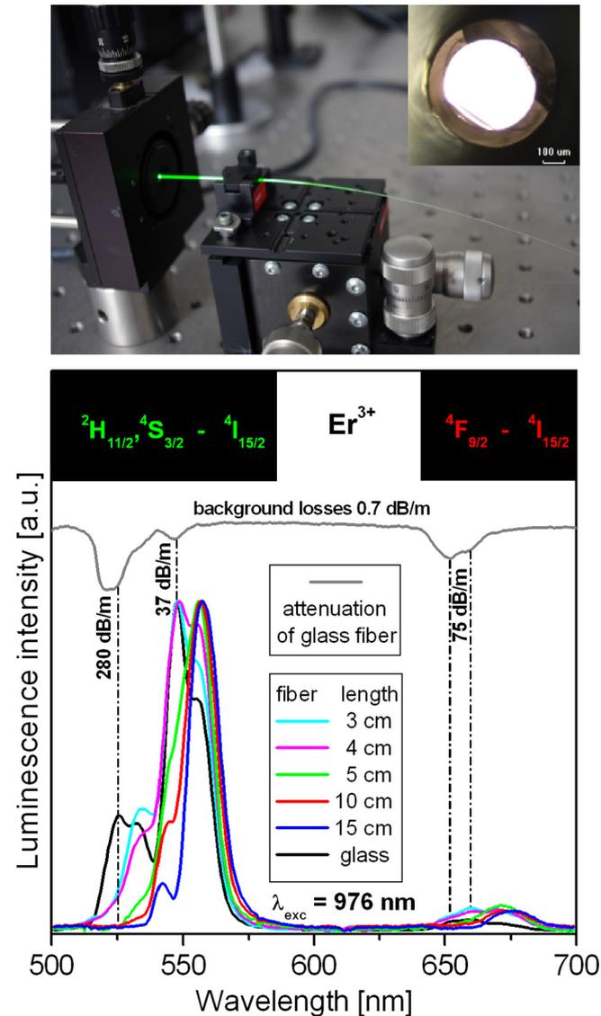
Fig. 1. Up-conversion emission of  $\text{Er}^{3+}$  in fibers (bottom). The inset shows the photo of green up-conversion emission and cross-section of the fabricated fiber (top).
