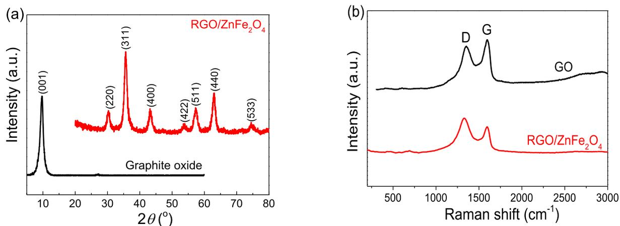
Fig. 1. (a) XRD patterns of graphite oxide and RGO/ZnFe<sub>2</sub>O<sub>4</sub> hybrid nanocomposite, (b) Raman spectra of GO and RGO/ZnFe<sub>2</sub>O<sub>4</sub> hybrid nanocomposite.
