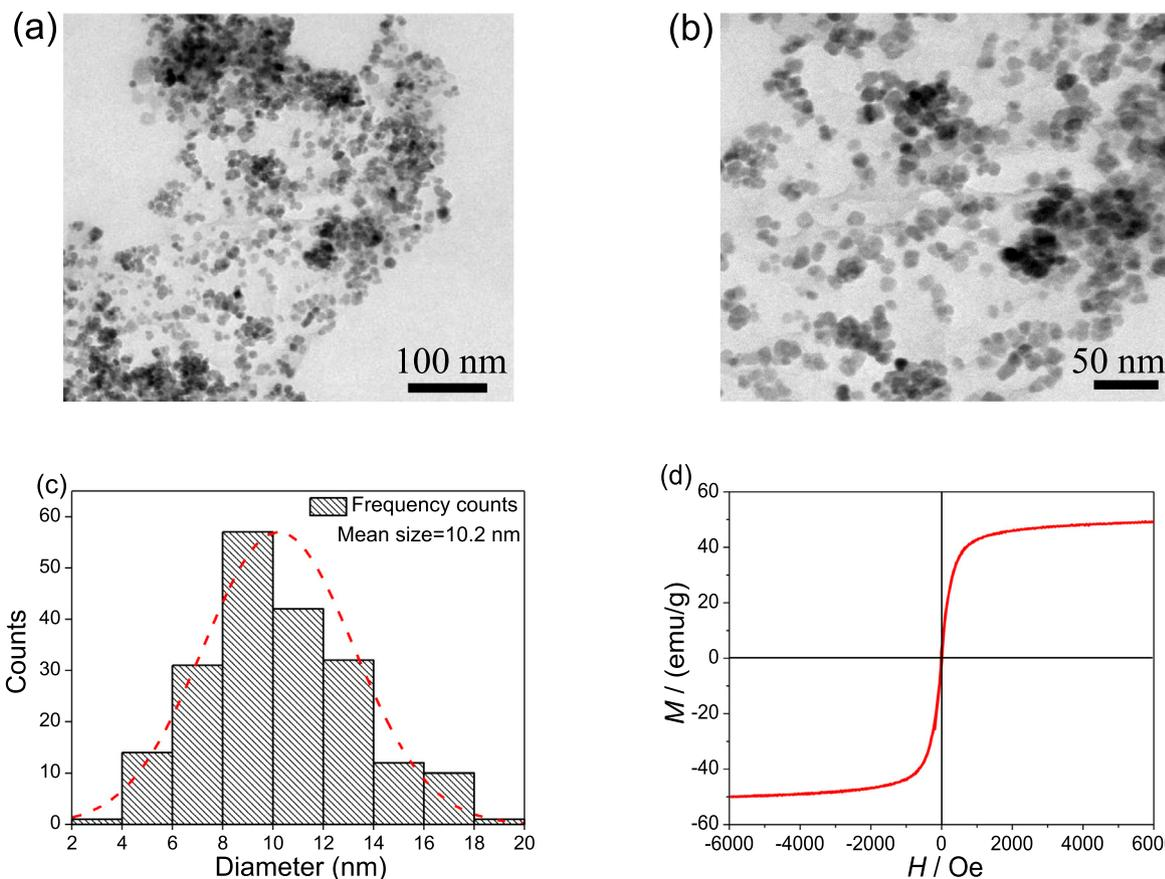
Fig. 2. (a)–(b) TEM images of RGO/ZnFe<sub>2</sub>O<sub>4</sub> hybrid nanocomposite with different magnifications, (c) particle size distribution histogram of ZnFe<sub>2</sub>O<sub>4</sub> nanoparticles and (d) magnetic hysteresis loop of RGO/ZnFe<sub>2</sub>O<sub>4</sub> hybrid nanocomposite.
